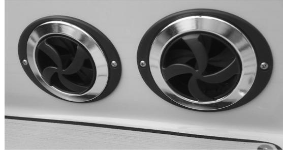
The boat heater is a forced air heater that uses hot engine water as a heat source. To use the heater, simply turn the heater switch to the selected fan speed. In order for the heater to work, the engine must be at operating temperature. One of the features of the heater are the snorkel vents, which can be pulled out to direct heat to specific areas.
