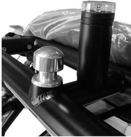
On boats equipped with factory installed towers, the 360° White Anchor/Running Light is mounted on the tower.
