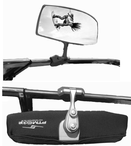
The rear view mirror is installed as a standard item. The mirror is adjustable so that it may be set for each driver.
