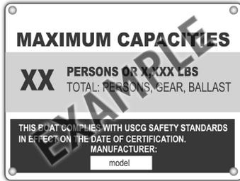
In compliance with United States Coast Guard Regulations, Moomba Boats meet or exceed all safety standards designed for recreational boats. To ensure safe handling and performance, each Moomba boat displays a maximum capacity sticker (see sample), stating the maximum passenger weight load allowable.
