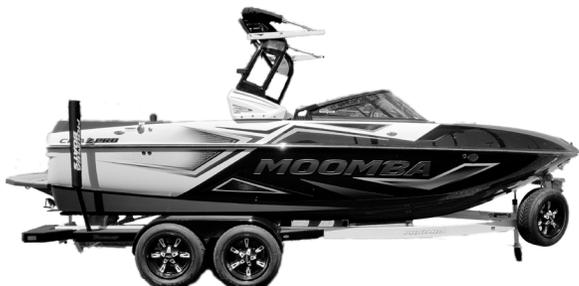
The trailer supplied with your Moomba model was designed especially for the boat with your convenience in mind. Please be sure that you have an appropriate tow vehicle before attempting to trailer your boat. Your vehicle must be capable of towing 4,500 — 6,000 lbs., depending on the model.
