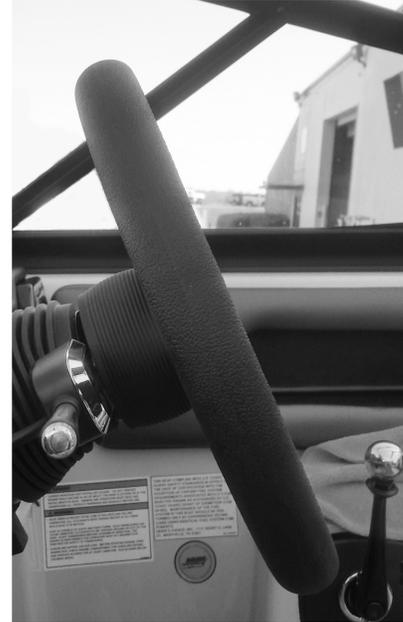
Tilt steering may be adjusted up or down in five different locking positions. To adjust, depress the tilt lever located beneath the bezel and move the steering wheel to the desired position. Release the lever to lock the wheel into place.
