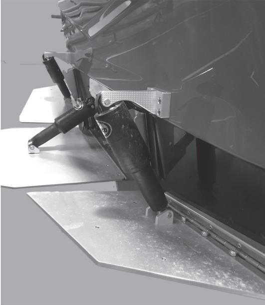
The multisport wakeplate allows the driver to control the running attitude of the boat.
