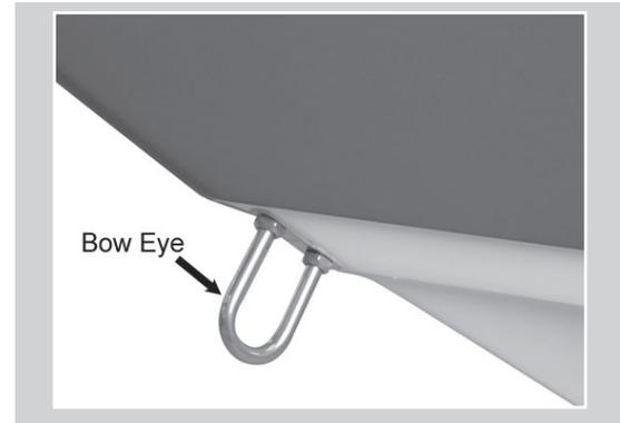
The bow eye is located at the front of the hull below the rub rail. It is the point of attachment to lead the boat onto the trailer and to secure the boat to the trailer or to a tie-off when docking.
