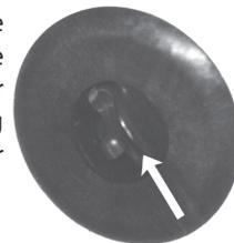
Inspect the paddlewheel and remove any foreign material only when engine is off.
