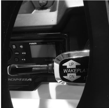
The Wakeplate switch controls the position of the center trim tab (wakeplate). The down position raises the stern of the boat and lowers the bow. The wakeplate helps shape the wake for surfing and wakeboarding.
