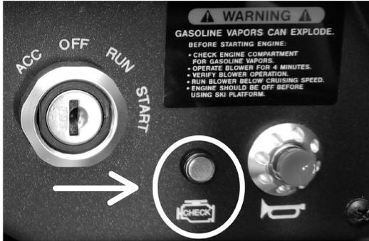
Your boat has an amber check engine light. It functions much the same as the check engine light in your car. If the engine control module senses certain engine parameters out of range a trouble code is set, and the light will come on.
