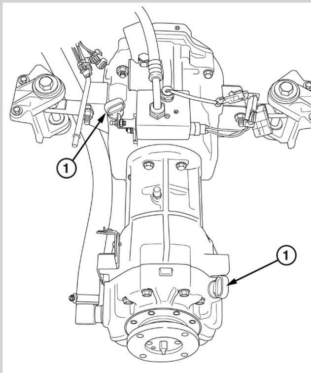
The fluid level can be checked by using the oil level dipstick, which is located on top of the V-Drive transmission. This unit's located under the center cushion of the rear seat. Pull out the cushion to access the transmission.
