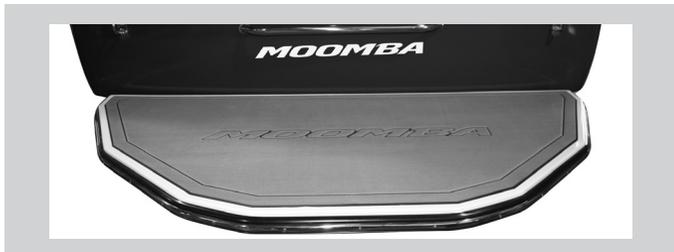
All Moomba models are equipped with a ski platform on the stern. The platform allows easy access to and from the water for skiers and swimmers. It is recommended that all entries to and exits from the water be made from the platform to avoid accidents. (The fiberglass deck can become slippery when wet.)
