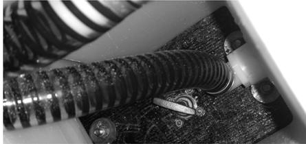
The center drain plug is accessed via the access cover in the center floor panel.
