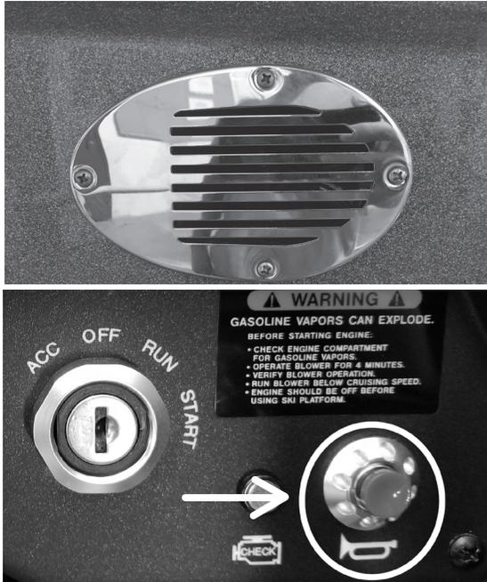
The Horn Switch is located on the switch panel to the left of the steering wheel.
