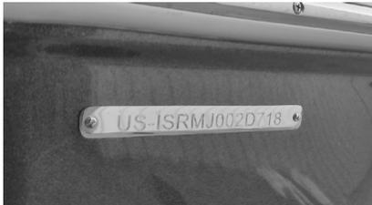
The hull identification number is located on the upper right hand side of the transom below the rub rail.
