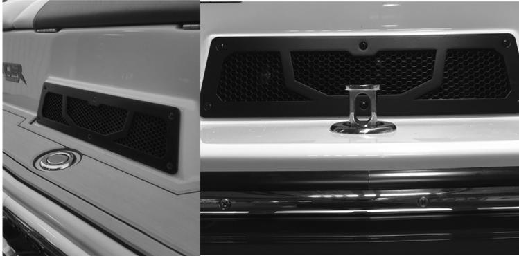
The ski pylon is only to be used to pull skiers. **DO NOT use the ski pylon to hoist the boat.** Only use the lifting rings for this purpose.
